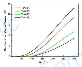
The chart for matched load output power Vs T<sub>h</sub> under various T<sub>c</sub>
