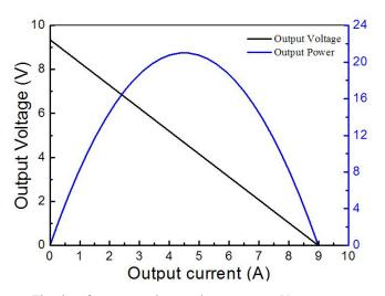
The chart for output voltage and output power Vs output current under T\_h=300  $^\circ C$  and T\_c=50  $^\circ C$
