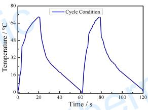
Typical cooling-heating cycle
