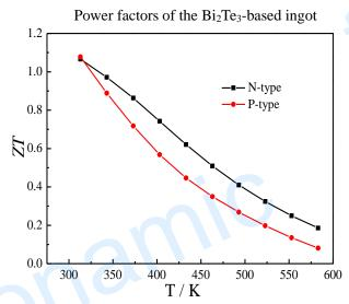
Z values of the Bi<sub>2</sub>Te<sub>3</sub>-based ingot
